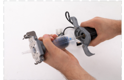
Pull the piston out from the syringe.
