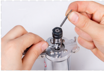
Take out the old cutter if any is inserted.
