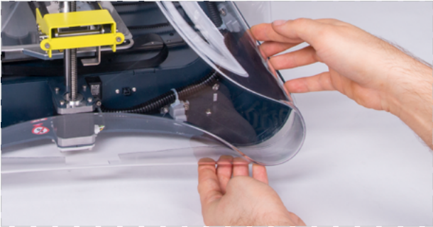
Pull out the cover rear corner from the machine frame.
