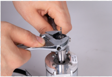
Adjust the size of wrench to 17 mm and hold down the collet fastening nut. Loosen the nut.
