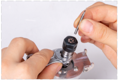
Put in a new cutter. Ensure that it is inserted at least 15 mm deep.
