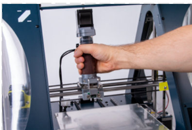
Put the Thick Paste toolhead on the X-carriage mount.
