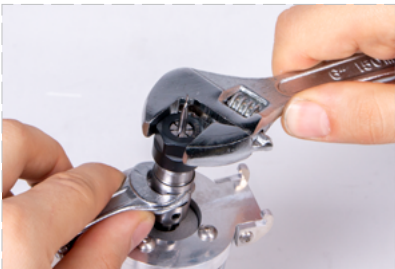
Firmly tighten the collet nut.
