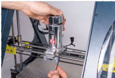
Mount the CNC toolhead on the X-carriage
