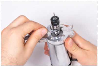
Slide the 13-mm spanner into the shown slot.
