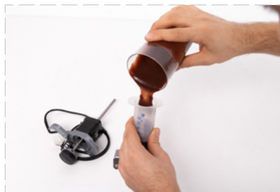
Fill the syringe with the prepared material.
