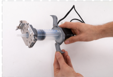
Unlock the syringe blockade.
