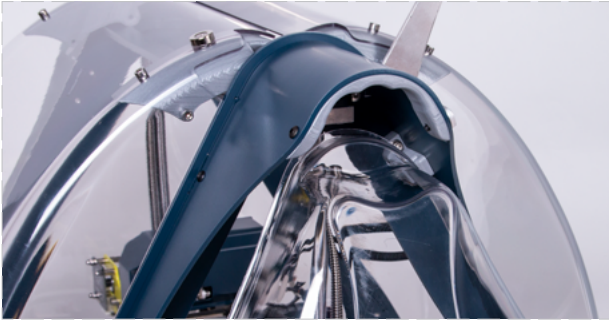
Pull out the cover upper corner from the machine frame.
