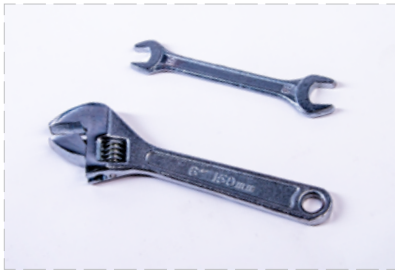
Take a 13 mm spanner and an adjustable wrench.
